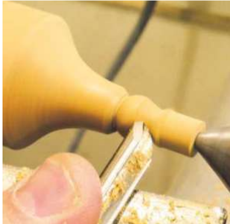
▲ Pic.20 Turn the end down to about 8mm, but leaving about 10mm waste on the end to be sure that you have removed the hole left by the centre
